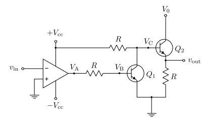
Assume that  $R = 10 \text{ k}\Omega$ ,  $V_{cc} = 15 \text{ V}$ , and  $V_0 = 5 \text{ V}$ . In this problem you are simply asked to complete the table shown below. For the input voltages  $v_{in}$  shown in the table, enter the resulting values for  $V_A$ ,  $V_B$ ,  $V_C$ , and  $v_{out}$ . In the  $Q_1$  and  $Q_2$  columns indicate whether each transistor is conducting or not conducting. If a transistor is in its conducting state, enter "ON". If a transistor is not conducting, enter "OFF".
