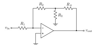
(a) Find an expression for the gain  $(G = v_{out}/v_{in})$  of the amplifier in terms of  $R_1$ ,  $R_2$ ,  $R_3$ , and  $R_4$ . (7 marks)
